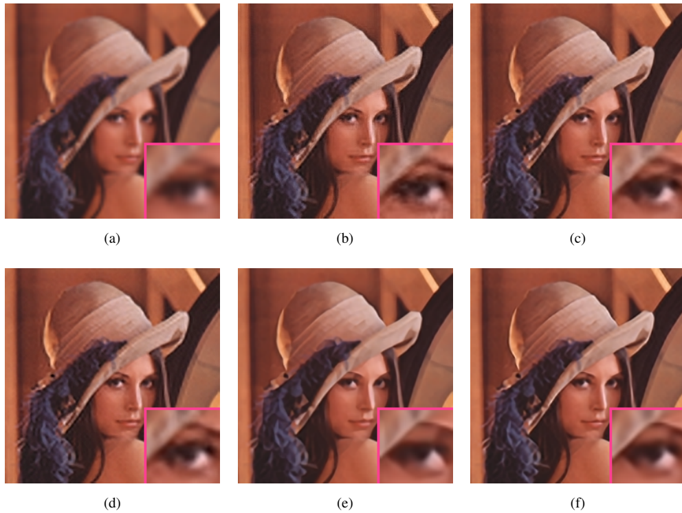
Fig. 10. Comparative results with zoomed-in areas for Lena magnified by a factor of 3. The methods considered are: (a) Bicubic interpolation, (b) LLE-based NE, (c) NN NE, (d) Sparse SR, (e) Pyramid, (f) Proposed.
