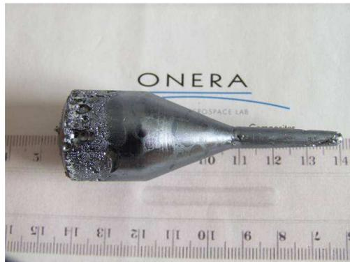
Figure 1: picture of a ZnGeP<sub>2</sub> crack free single crystal
