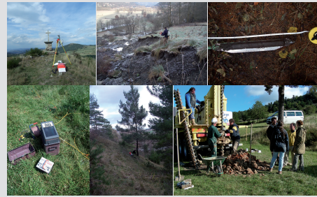
Figure 2 – Example of field investigation (DGPS monitoring, peat extraction for C14 datation, geophysics, Pressler extraction on a tree, borehole)
