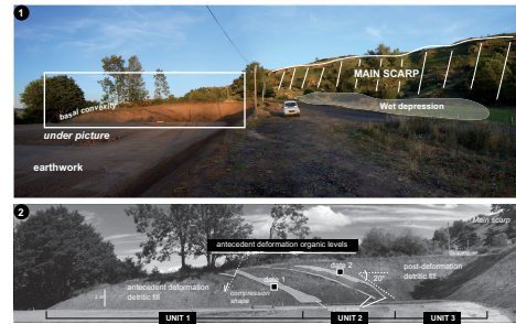
Figure 4 – Example of a palaeolandslide. 1) general context of the landslide; 2) details of the formations and the mechanic deformation of detritic and organic filling
