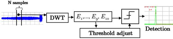
Figure 3. Flowchart of the wavelet based algorithm
