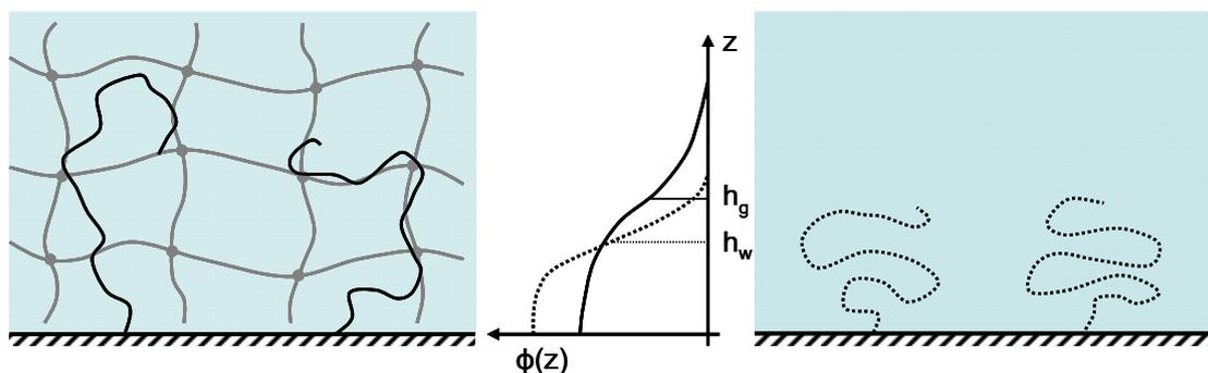
**Figure 4.** Schematic representation of the brush structure against the gel and against water at pH 2. The brush is more extended in the presence of the gel at pH 2 when there are specific interactions between the gel and the brush with hydrogen bonds.  $h_g$  and  $h_w$  are the mean heights of the brush in the presence of the gel, and in water respectively.
