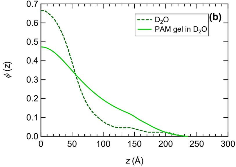
**Figure 3.** (a) Neutron reflectivity curves and (b) polymer volume fraction profiles corresponding to the best fit of the reflectivity data. Experiments are carried out with the PAA brush at pH 2, in D<sub>2</sub>O (dark green and dashed line) or in contact with a PAM gel (light green and solid line). The reflectivity curves are shifted vertically for clarity.
