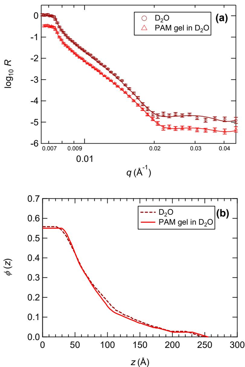
**Figure 2.** (a) Neutron reflectivity curves and (b) polymer volume fraction profiles corresponding to the best fit of the reflectivity data. Experiments were carried out with the PAA brush at pH 9, in D<sub>2</sub>O (dark red and dashed line) or in contact with a PAM gel (light red and solid line). The reflectivity curves are shifted vertically for clarity.
