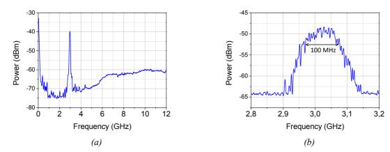
**Fig. 7.** Beat note analysis with an 18 GHz electronic spectrum analyser. The spectra shown are envelope of multiple scans accumulated over 20 s.
