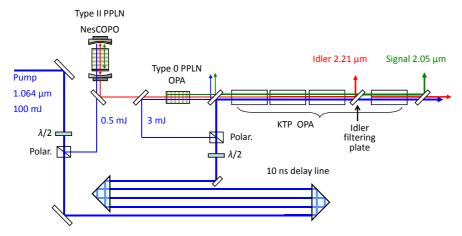
**Fig. 2.** Experimental set-up for the high energy MOPA. The wavelengths represented correspond to the case where the signal is emitted in the CO<sub>2</sub> R30 line around 2051 nm.
