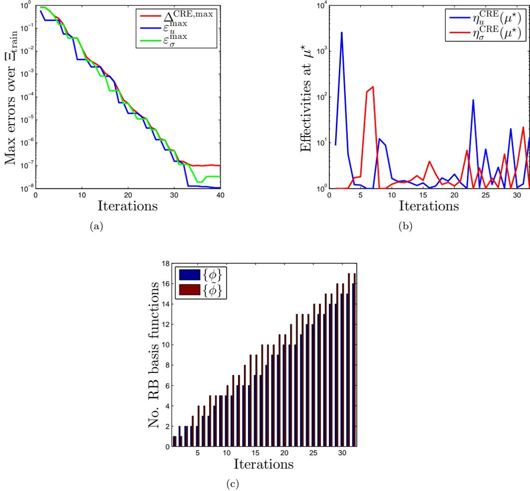
Figure 5: (a) Maximum of CRE error  $\Delta^{\text{CRE,max}}$ , displacement RB error  $\varepsilon_u^{\text{max}}$  and stress RB error  $\varepsilon_\sigma^{\text{max}}$  over  $\Xi_{\text{train}}$ , (b) displacement and stress effectivities at  $\mu^*$ , and (c) sizes of the sets  $\mathcal{Z}_N$  and  $\tilde{\mathcal{Z}}_N$  as functions of Greedy iterations (only first 32 iterations are shown in fig. 5(b) and fig. 5(c)).
