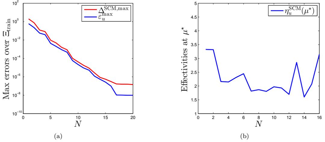
Figure 6: (a) Maximum of SCM upper error bound  $\Delta^{\text{SCM,max}}$  and displacement RB error  $\varepsilon_u^{\text{max}}$  over  $\Xi_{\text{train}}$ , and (b) displacement effectivity at  $\mu^*$  as functions of  $N$  (only first 16 iterations are shown in fig. 6(b)).
