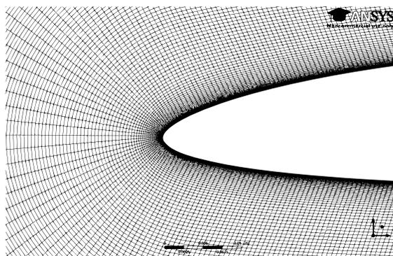
Figure 3: High-density mesh close to the leading edge
