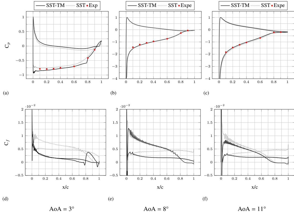
Figure 14: Pressure and friction coefficients at  $AoA = 3^\circ$  ((a) and (d)),  $8^\circ$  ((b) and (e)) and  $11^\circ$  ((c) and (f)),  $Re = 7.5 \times 10^5$
