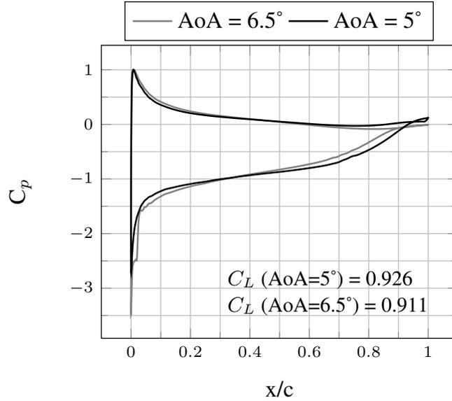
Figure 8: Pressure coefficient distribution at AoA = 5° and AoA = 6.5°,  $Re = 7.5 \times 10^5$
