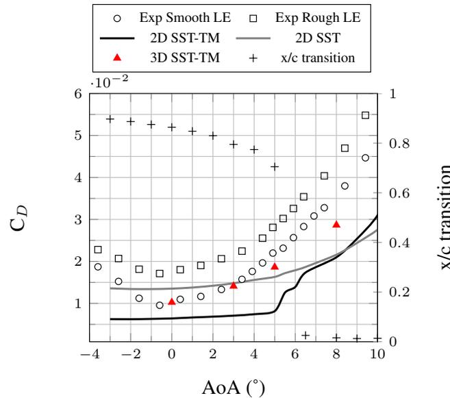
Figure 9: Experimental vs numerical drag coefficients, zoom of Figure 7 (b),  $Re=7.5 \times 10^5$  (the reader is referred to the web version of this article for an easier understanding of this figure: 3D marks are red triangles).
