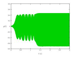
(a) Pressure signal for the light grey (orange in colored version) point 1 (see Fig. 8) ( $\gamma = 0.424, \zeta = 0.240$ )
