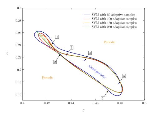
**Fig. 8:** Focus on the boundary between periodic and quasi-periodic regimes according to the number of adaptive points used. Samples have been omitted for sake of readability. The pressure signals represented by the points 1 to 6 are plotted on the Figure 9.
