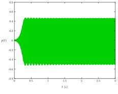
(f) Pressure signal for the light grey (orange in colored version) point 6 (see Fig. 8) ( $\gamma = 0.470, \zeta = 0.170$ )
