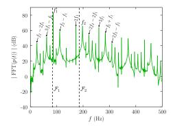
(a) Spectrum of a quasi-periodic signal whose descriptor  $\epsilon$  is equal to  $4.10^{-1}\%$  (black/blue dot from Figure 4).  $f_1$  and  $f_2$  are two incommensurate frequencies whose linear combinations correspond to the peaks frequencies in the spectrum.
