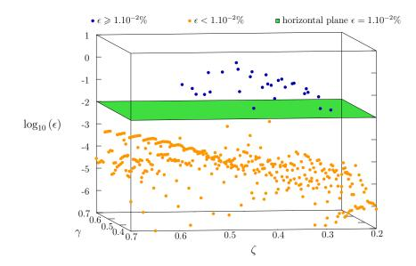
**Fig. 4:** Descriptor  $\epsilon$  (see Eq. (10)) calculated on the mouthpiece pressure signal for a regular mesh of the control parameters space (inharmonicity is set to  $\Delta f/f = 150\%$  and  $\epsilon$  is expressed as a percentage).
