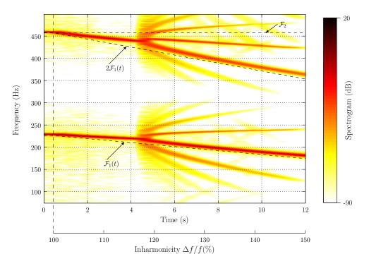
Fig. 12: Time-frequency representation of a pressure signal simulated for a variable inharmonicity over time. The inharmonicity increases linearly from the value  $\Delta f/f = 100\%$  to  $\Delta f/f = 150\%$ . The control parameters are fixed:  $\gamma = 0.47$  and  $\zeta = 0.28$ .  $\mathcal{F}_1$  and  $\mathcal{F}_2$  are the first and second resonance frequencies respectively of the dynamical system (8).
