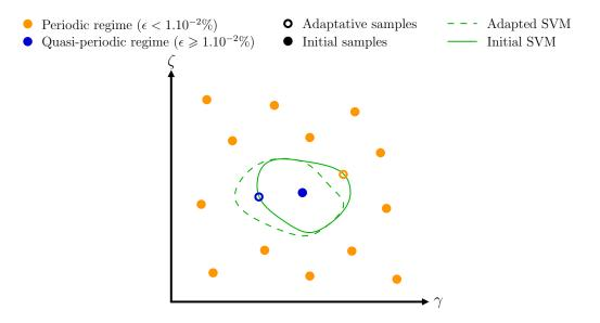
**Fig. 6:** Schematic representation of the EDSD adaptive sampling scheme. The addition of samples (circles) in the sparse region of the space on the SVM is the basis of EDSD. The dashed boundary corresponds to the updated SVM.
