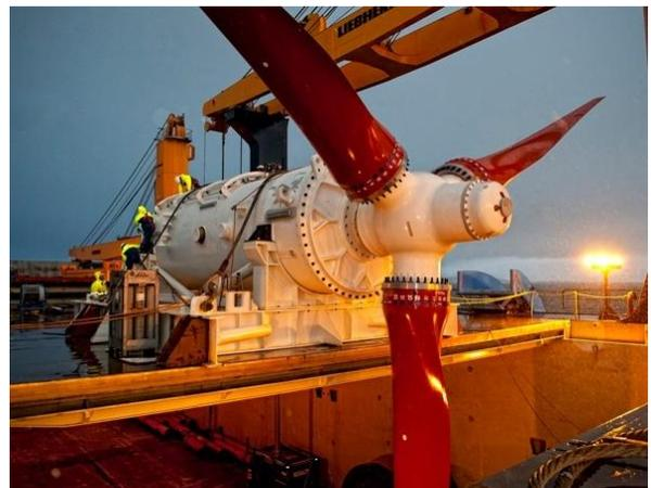
Fig. 2. Andritz Hydro Hammerfest HS1000 turbine © [12].
