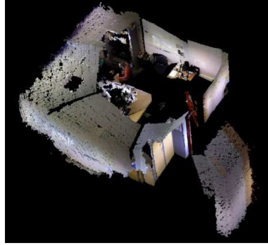
Figure 3: Point cloud obtained from the spherical RGBD acquisition system.
