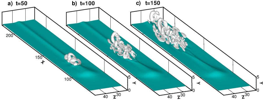
FIGURE 19. Surface of the instantaneous streamwise velocity  $u = -0.2$  and of the Q-criterion (light gray for  $Q = 100$ ) extracted by a DNS initialized by the optimal perturbation obtained for  $Re = 300$ ,  $k = 1.5$ ,  $T = 50$  with initial energy  $E_0 = 0.001$  at  $t = 50$  (a),  $t = 100$  (b),  $t = 150$  (c.)
