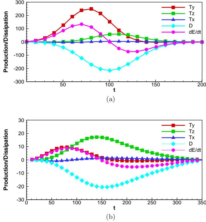
FIGURE 13. Perturbation kinetic energy time derivative, and production and dissipation terms versus time extracted by a linearized DNS initialized by the VP\* (a) and the SP\* (b).
