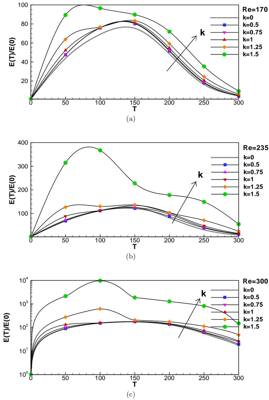
FIGURE 4. Optimal energy gain versus target time for the Blasius base flow (dotted line) and in the presence of the bumps of different heights (increasing bump height following the arrow), for  $Re = 170$  (a),  $Re = 235$  (b), and  $Re = 300$  (c). The symbols correspond to:  $k = 0.5$  (squares),  $k = 0.75$  (gradients),  $k = 1$  (deltas),  $k = 1.25$  (diamonds), and  $k = 1.5$  (circles).
