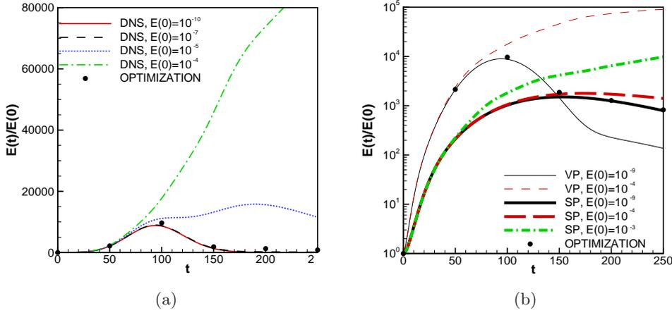
FIGURE 16. Energy gain versus time extracted by a DNS initialized by the optimal perturbation obtained for  $Re = 300$ ,  $k = 1.5$ ,  $T = 50$  (VP\*, left frame) and  $T = 200$  (SP\*, right frame) with the initial energies indicated within the figure. The black dots indicate the optimal energy gain obtained at target time by the linear optimization.
