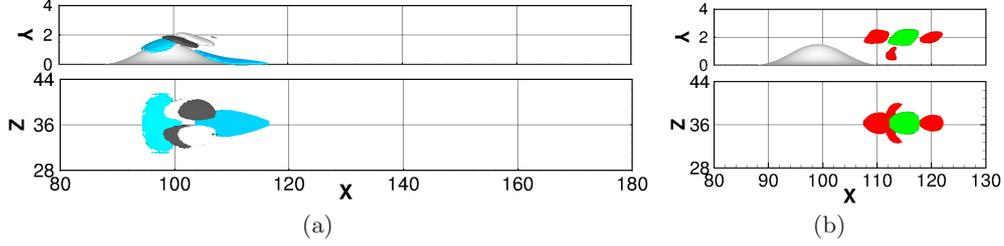
FIGURE 14. Base flow shear (grey, blue online), streamwise vorticity perturbation (white and black for  $\omega_x = \pm 0.001$ ) at  $t = 0$  (a) and streamwise velocity perturbation (dark grey, red online, and light grey, green online, for  $u' = \pm 10^{-5}$ ) at  $t = 25$  (b) for the optimal perturbation obtained for  $Re = 300$ ,  $k = 1.5$ ,  $T = 50$ .
