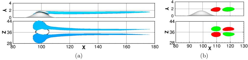
FIGURE 15. Base flow shear (grey, blue online), streamwise vorticity perturbation (white and black for  $\omega_x = \pm 0.001$ ) at  $t = 0$  (a) and streamwise velocity perturbation (dark grey, red online, and light grey, green online, for  $u' = \pm 10^{-5}$ ) at  $t = 25$  (b) for the optimal perturbation obtained for  $Re = 300$ ,  $k = 1.5$ ,  $T = 200$ .
