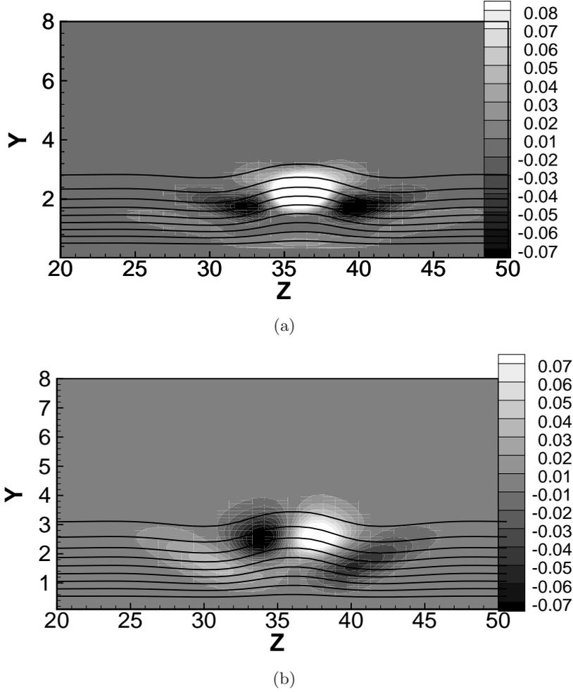
FIGURE 10. Shaded contours of the streamwise velocity component of the optimal perturbation at target time  $T = 100$  (a) and  $T = 150$  (b) in the planes  $x = 135$  (a) and  $x = 165$  (b) with  $Re = 235$  and  $k = 1.5$ . The solid contours represent the streamwise component of the base flow velocity in the range  $[0.1, 0.9]$ . Axis are not on the same scale.
