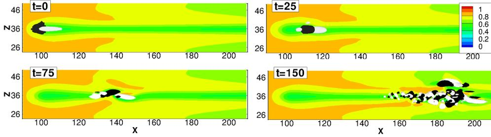
FIGURE 18. Contours of the instantaneous streamwise velocity at  $y = 2$  and surfaces of the streamwise vorticity perturbation (white and black) extracted by a DNS initialized by the optimal perturbation obtained for  $Re = 300$ ,  $k = 1.5$ ,  $T = 200$  with initial energy  $E_0 = 0.01$  at  $t = 0$ ,  $t = 25$  (surfaces for  $\omega_x = \pm 0.015$ , first and second frame, respectively),  $t = 75$  and  $t = 150$  (surfaces for  $\omega_x = \pm 0.1$ , third and fourth frame, respectively).
