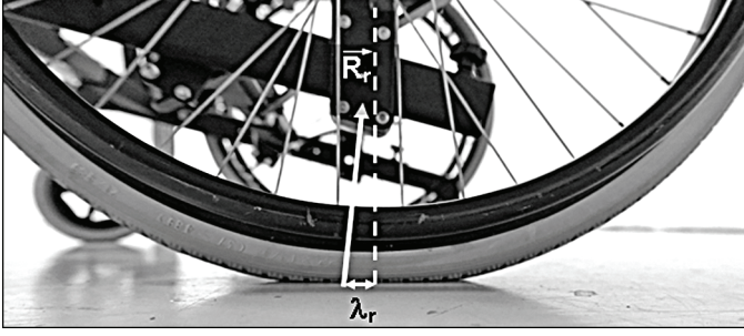
Figure 1. Representation of rear wheel rolling resistance parameter, which is fore-aft length between theoretical and real centers of pressure during rolling. \overline{R}_r is ground reaction force applied on rear wheel.
