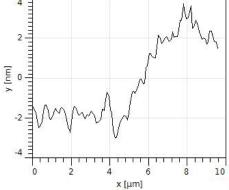
**Figure 6**: AFM images of a step created by O<sub>2</sub> plasma etching on weakly N-type polySi and step measurement of the grafted surface.
