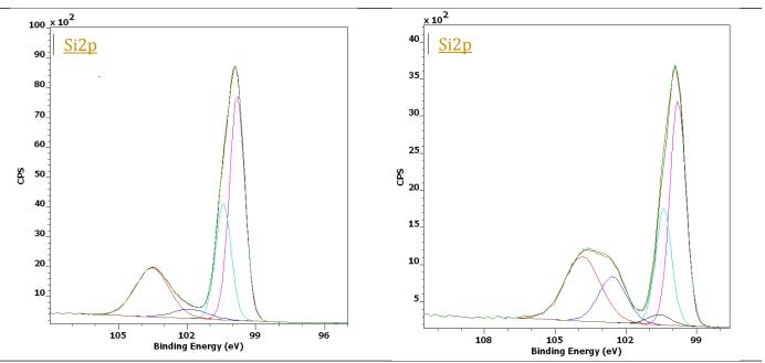
Figure 4: Deconvolution of C1s and Si2p core level spectra obtained with AlKa excitation
