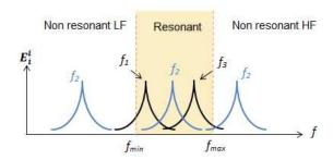
Figure 5 – Sketch of the natural frequencies of each oscillator. The resonance frequency of oscillator 2 varies.
