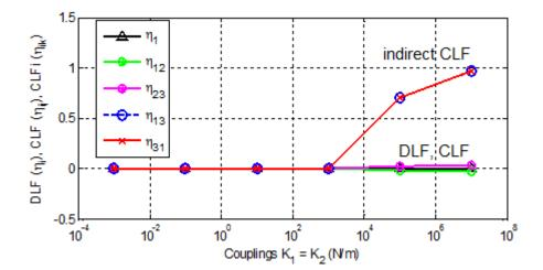
Figure 4 – Evolution of the CLF, DLF and CLFi versus the couplings stiffness  $K_1 = K_2$  with large bandwidth.
