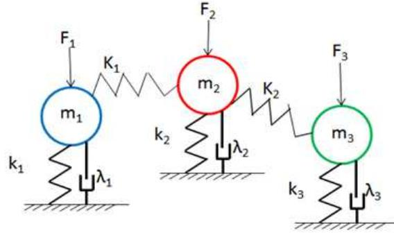
Figure 1 – Three oscillators excited by uncorrelated random forces  $F_i$  coupled by elastic couplings  $K_i$ .
