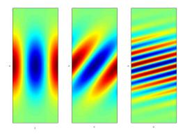
Figure 1: Damping of an initial spatial structure by free transport (periodic spatial boundary condition are used). Left = initial condition; Center and Right: the shear in phase space creates finer and finer structures. After integration over the v variable, the spatial structure damps.
