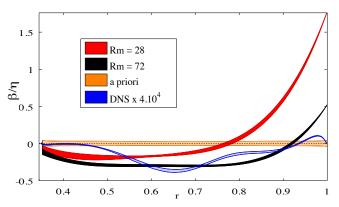
FIG. 2. Radial profiles of the  $\alpha$ -effect (a) and  $\beta$ -effect (b) with their error bars, obtained by the inversion of DTS data for two magnetic Reynolds number: Rm=28 and 72. The *a priori* null profile, along with its error bar, is also drawn. The blue curve shows the  $\alpha(r)$  and  $\beta(r)$  profiles retrieved from a numerical simulation of the DTS experiment at Rm=29 and  $Re=2.9\times10^4$ , blown up by a factor  $4\times10^4$ .
