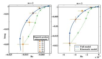
FIG. 3. Measurements and model fits for an example of time-varying magnetic signals measured at 2f (m=2) and 3f (m=3) frequencies, for a rotation rate of the inner sphere f = -23Hz (Rm = 72). See text for explanations.
