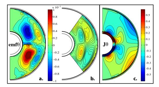
FIG. 4. Meridional cross section contour maps showing orthoradial component  $(\theta)$  of emf  $\mathcal{E}$  and of electrical current  $\langle \mathbf{J} \rangle$ . (a) Averaged emf  $\mathcal{E}_t$  obtained from DNS. (b) Reconstructed emf  $\mathcal{E}_{\alpha\beta}$  from inverted  $\alpha$  and  $\beta$  profiles. High latitudes (white area) are excluded from the least-square fit. (c) Mean electrical current from DNS.
