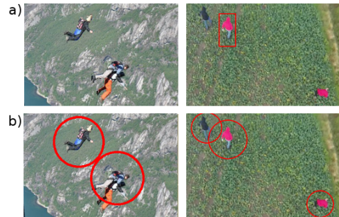
Fig. 1. a) results obtained with the ICF detector [1] b) and with the PRD: the detector is less sensitive to changes of shape and angle.
