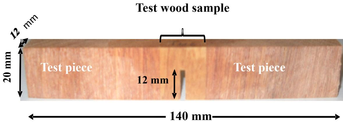
Figure 5 – Specimen for fracture energy test.
