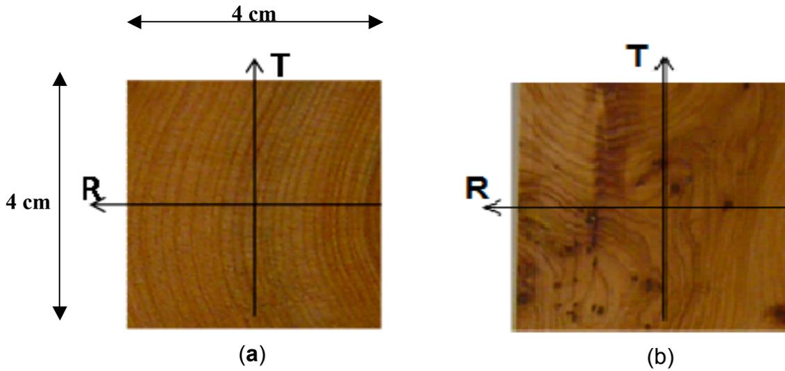
**Figure 2** - Cross-section of the material: (a) thuya wood; (b) thuya burl
