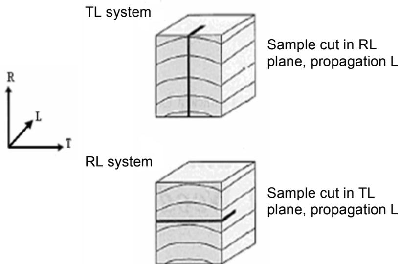
Figure 6 Fracture system notation (illustrated for wood)
