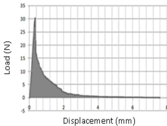
**Figure 8** – Example of force - displacement curve (thuya wood, TL system).
