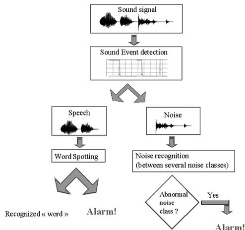
The sound classification method uses a Gaussian Mixture Model (GMM), with 4 gaussian components. The sound recognition system was tested on a 7 classes test sets : dishes sound, door clapping, door lock, glass breaking, screams, telephone ringing and step sound. The best results are obtained with  $\Delta, \Delta\Delta$  MFCC parameters and the error rate is about 8.7% in average for all classes
