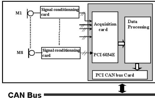
When a sound event is detected, the smart audio sensor sends a frame of information on the CAN bus. The frame contains: date and time detection (day, month, year, hour, minute, seconde, milliseconds), a flag to indicate the type of sound event (speech or noise) and a character field. This character field is composed by: the three most probable noise classes (or words) with their corresponding likelihoods and the localization of the sound event (the room).
