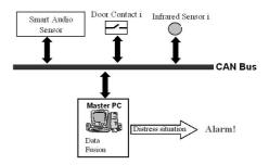
Figure 5: Hardware configuration
