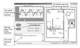
Figure 7: The panel of the real-time analysis software
