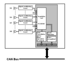
Figure 1: Smart Audio Sensor Diagram
