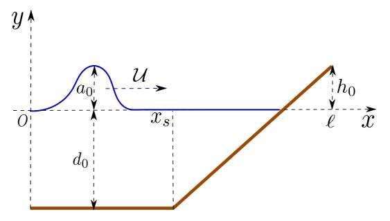
**Figure 5.** Sketch of the physical domain corresponding to our numerical simulations of a solitary wave run-up onto a plane beach [36].
