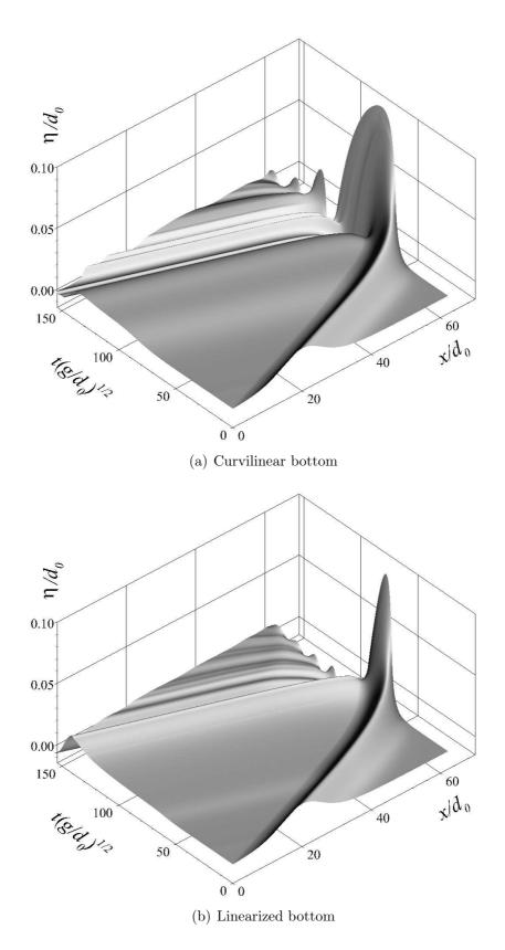
**Figure 11.** Space-time plots of the free surface evolution for  $a_0/d_0 = 0.02$  and  $\theta = 5^{\circ}$  for the curvilinear (a) and corresponding linearized (b) bottom profiles.
