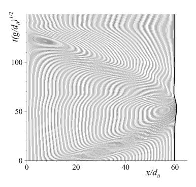
**Figure 7.** Trajectories of grid points during a solitary wave run-up with  $\theta = 2.88^{\circ}$  and  $a_0/d_0 = 0.01$ . Only every  $10^{\text{th}}$  point is shown for the sake of clarity. This computation corresponds to the space-time evolution shown on Figure 6. The black solid line shows the discrete trajectory of the shoreline point  $\{x_N^{(n)}\}$ .
