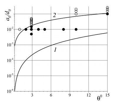
**Figure 8.** Applicability range of formula (5.2) bounded from below by condition (5.3) and from above by the wave breaking criterium (5.4). Numerical experiments which lie in the range of applicability of (5.2) are shown with filled circles  $(\bullet)$ . All the others, which are outside, are shown with empty circles  $(\circ)$ .
