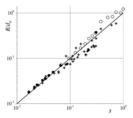
**Figure 9.** Comparison of maximal run-up values with the experimental data (+) [37] and the analytical prediction (5.2) (straight solid line). The horizontal variable S denotes the right hand side of the equation (5.2).
