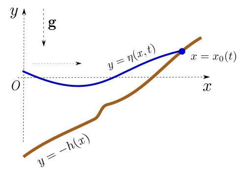
**Figure 1.** Sketch of the physical domain, where y = -h(x) is the bottom shape,  $y = \eta(x,t)$  is the free surface and  $x = x_0(t)$  is the moving shoreline. The horizontal blue dotted arrow shows the wave propagation direction.
