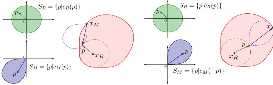
**Fig. 1. Non-overlapping constraint.** *Left:* two objects  $S_R$  and  $S_M$ , the region in red represents the set of all positions  $x_M$  for  $S_M$  that violate the non-overlapping constraint. *Right:* two objects  $S_R$  and  $-S_M$  and their Minkowski sum, which coincides with the overlapping constraint (the negation of the non-overlapping constraint).
