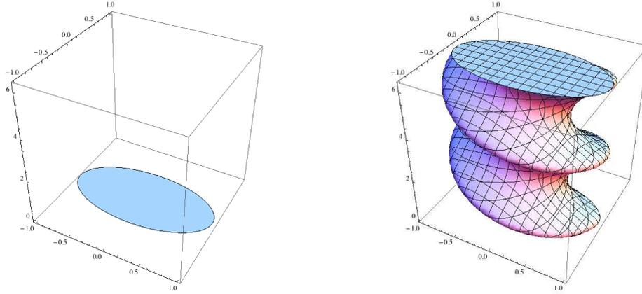
**Fig. 3.** Sets whose Minkowski difference gives the overlapping constraint of two ellipses, when rotation is taken into account. *Left:* the augmented reference ellipsoid, with rotation coordinate set to 0. *Right:* the augmented moving ellipsoid  $S'_M$ .
