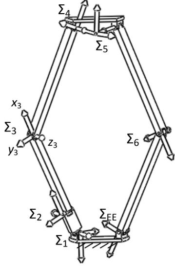
(a) Coordinate frame system for the SLR7RMMOM
