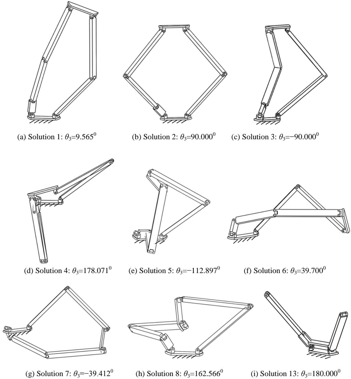
Fig. 5. CAD configurations corresponding to the real solutions
