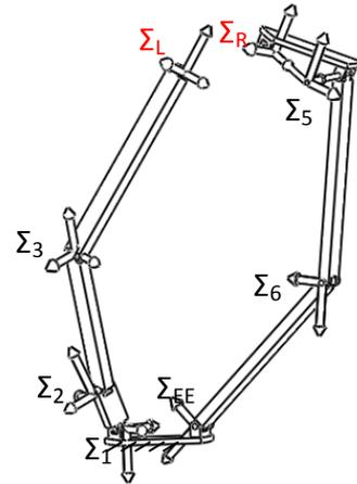
Fig. 4. Decomposing the loop into two 3R chains
