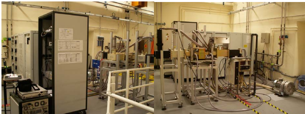
Figure 2.3: View of the RF Power supply setup at Orsay: on the left, the DC power generator as well as the 1 kW amplifier, the interlocks and control closet; on the right, a back view of the IOT with its circulators and all the pipes circuits for air and water cooling.
