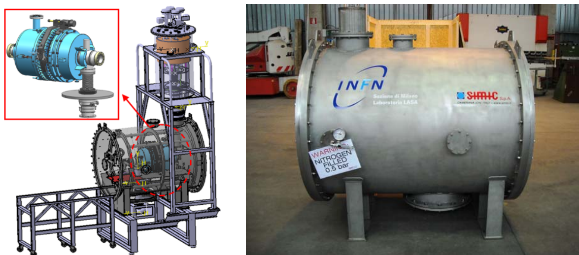
Figure 10.1.4: (left) scheme of the prototypical 700 MHz cryomodule, with its dressed cavity inside. (right) The module after vacuum leak tests at the SIMIC company.
