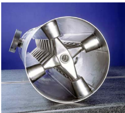
Figure 10.1.2: (left) the superconducting CH-prototype before the final welding. (right) measurement of the Q-value as function of the accelerating gradient.
