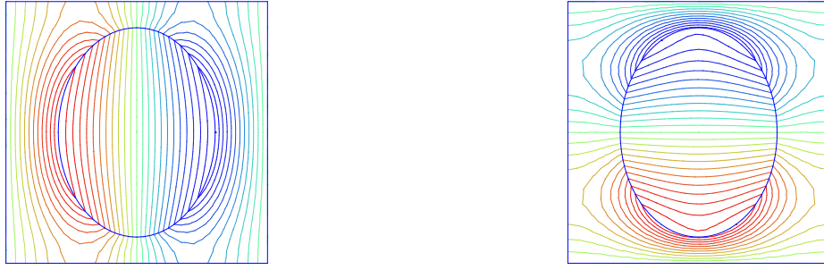
Figure 11.2: Potentials V_x (left) and V_y (right): The unit cell contains an elliptic inclusion of relative permittivity ( \varepsilon = 4.0 + 3i ) with minor and major axis a = 0.3 and b = 0.4 in silica ( \varepsilon = 1.25 ).
