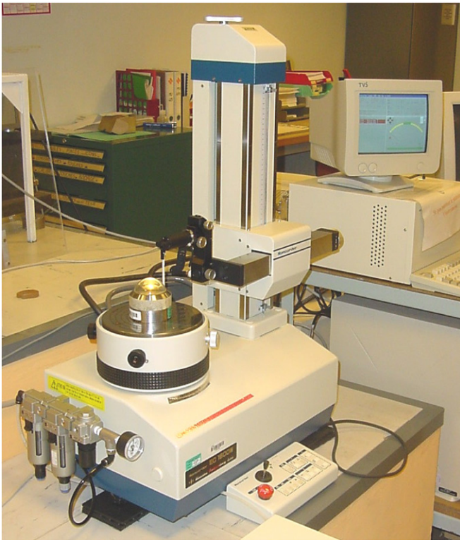
Figure 3. Example of a conventional geometry measurement machine: the KOSAKA machine.
