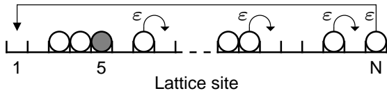
FIG. 1. TASEP model with pausing. (A) Particles can transition from an active state (in white) to a paused state (in grey) and back, with respective rates f and 1/\tau . (B) Active particles can hop to the next site if it is empty (exclusion process), with unit-time probability \epsilon . Paused particles do not move.
