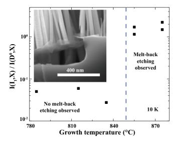
FIG. 2. (Color online) Evolution of the intensity ratio of the transitions from excitons bound to  $I_1$  stacking faults and neutral donors  $[I_{(I_1,X)}/I_{(D^0,X)}]$  at 10 K with growth temperature. The dashed line indicates the growth temperature above which Si melt-back etching is systematically observed. The inset shows a cross-sectional scanning electron micrograph of a pit caused by the melt-back etching of the Si substrate.
