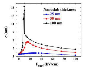
FIG. 7. (Color online) Standard deviation of the electron position  $\sigma$  as a function of the surface electric field  $F_{\rm surf}$  for three nanoslab thicknesses d.
