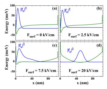
FIG. 6. (Color online) Effective potential (green solid line) and probability distribution  $|f_e|^2$  (blue solid line) for an electron in a GaN nanoslab with a thickness of 100 nm and for a surface electric field  $F_{\rm surf}$  of 0 (a), 2.5 (b), 7.5 (c), and 20 kV/cm (d). The donor is located at the left surface of the nanoslab. The y scale for  $|f_e|^2$  is shown in arbitrary units.
