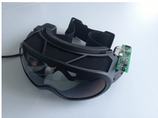
Fig. 11. Marine Mobile Augmented Reality System (first prototype)
