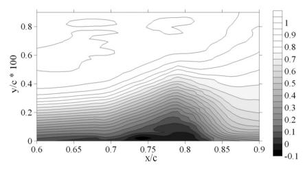
**Fig. 8.** Laminar Separation Bubble near the trailing edge: isovalues of the longitudinal velocity component  $u/u_{\rm ext}$  through the boundary-layer for  $\alpha=2^{\circ}$  and Re=750 000.
