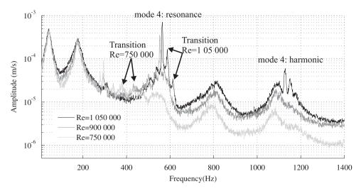
**Fig. 18.** Comparison of flexible hydrofoil velocity spectra for  $\alpha = 4^{\circ}$  and various Reynolds numbers.
