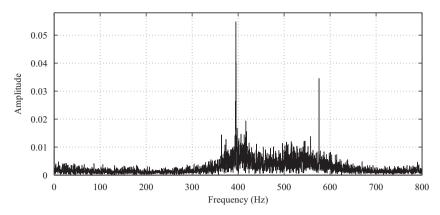
**Fig. 11.** Frequency spectra of the wall pressure fluctuations at x/c=0.8 for  $\alpha=2^{\circ}$  and Re=750 000.
