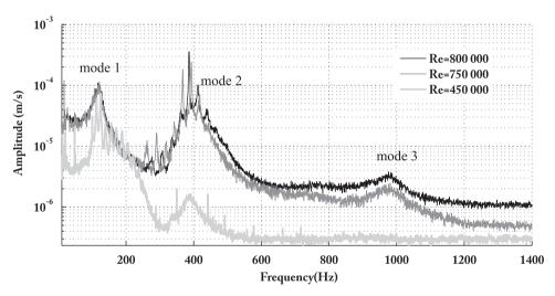
**Fig. 15.** Rigid hydrofoil, velocity spectra for  $\alpha = 4^{\circ}$  and various Reynolds numbers.
