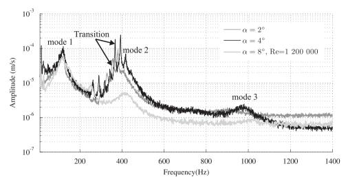
**Fig. 14.** Rigid hydrofoil, normal velocity spectra for  $\alpha = 2$ ,  $\alpha = 4^{\circ}$  at Re=750 000 and  $\alpha = 8^{\circ}$  at Re=1 200 000.
