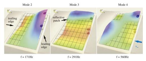
Fig. 16. Experimental mode shapes of the flexible hydrofoil obtained from scanning measurements at the grid points.
