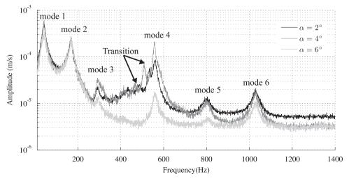
**Fig. 17.** Flexible hydrofoil normal velocity spectra for  $\alpha = 2^{\circ}$ ,  $\alpha = 4^{\circ}$  and  $\alpha = 6^{\circ}$ , Re=800 000.
