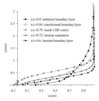
**Fig. 4.** Mean velocity profiles from x/c=0.6 to x/c=0.9 for  $\alpha=2^{\circ}$  and Re=750 000.
