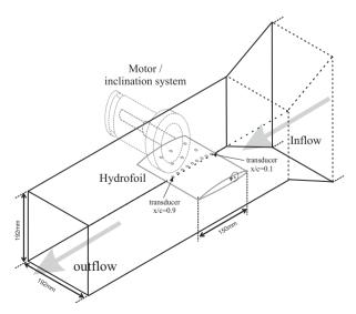
Fig. 1. Experimental set-up, rigid hydrofoil.
