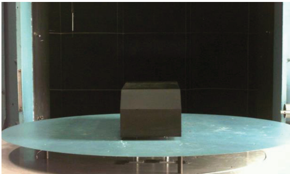
Fig. 1 Wind tunnel test section with Ahmed body
