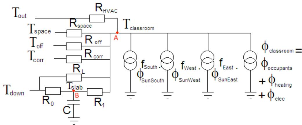
Figure 2 - equivalent electrical circuit of the classroom[CS1]
