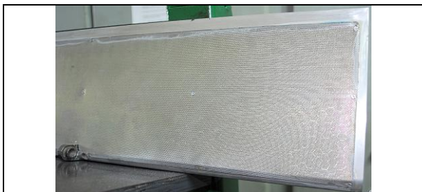
Figure 19: Lined flap model used in the experimental campaign.
