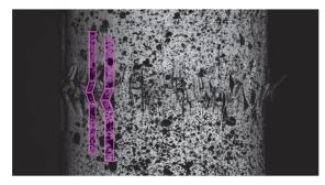
(b) Microbuckling of the tows (case d~0.95)
