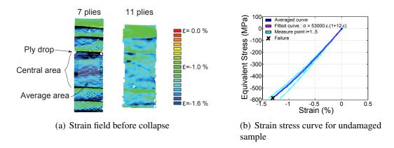
Figure 5. Strain for undamaged sample just before rupture
