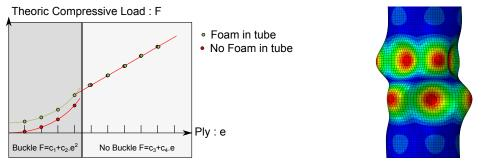
(a) Theorical compressive load for material or buckle (b) Visualization of the shell buckle in the central collapse area
