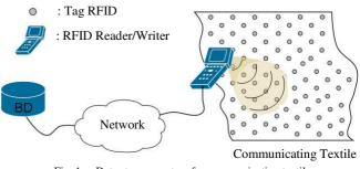
Fig. 1. Data storage system for communicating textile.
