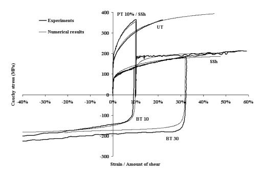
UT stands for Uniaxial Tension, BT for Bauschinger Test, SSh for Simple Shear and PT 10% SSh for Plane Tension until 10% of logarithmic strain followed by Simple Shear.
