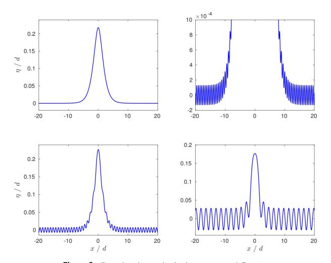
Figure 3. Examples of generalised solitary waves with  $Fr_0 = 1.1$ . Up-left:  $Bo_0 = 0.1$ ,  $Bo_\infty = 0.0999998$ ,  $Fr_\infty = 1.099999$ ; Up-right: zoom of up-left; Low-left:  $Bo_0 = 0.15$ ,  $Bo_\infty = 0.1499$ ,  $Fr_\infty = 1.099$ ; Low-right:  $Bo_0 = 0.25$ ,  $Bo_\infty = 0.248$ ,  $Fr_\infty = 1.095$ .
