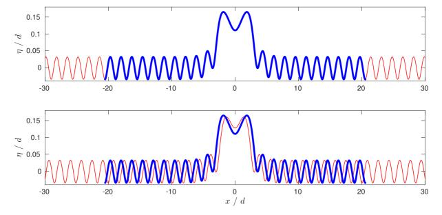
Figure 5. Influence of the computational box for  $Fr_0 = 1.1$  and  $Bo_0 = 0.25$ . Thick blue line:  $\Lambda/d_0 = 20$ ,  $d_\infty/d_0 = 1.00914$ ,  $Fr_\infty = 1.0873$ ,  $Bo_\infty = 0.24549$ ; Upper thin red line:  $\Lambda/d_0 = 30.11$ ,  $d_\infty/d_0 = 1.00913$ ,  $Fr_\infty = 1.0874$ ,  $Bo_\infty = 0.2455$ ; Lower thin red line:  $\Lambda/d_0 = 30.5$ ,  $d_\infty/d_0 = 1.0095$ ,  $Fr_\infty = 1.0868$ ,  $Bo_\infty = 0.24531$ .
