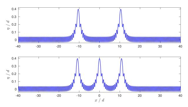
Figure 6. Multi-hump generalised solitary waves with  $\text{Fr}_0 = 1.17$  and  $\text{Bo}_0 = 0.12$ . Upper:  $\text{Fr}_{\infty} = 1.2466$ ,  $\text{Bo}_{\infty} = 0.1181$ ,  $d_{\infty}/d_0 = 1.008$ ,  $\max(\eta/d_{\infty}) = 0.4018$ . Lower:  $\text{Fr}_{\infty} = 1.2396$ ,  $\text{Bo}_{\infty} = 0.1183$ ,  $d_{\infty}/d_0 = 1.007$ ,  $\max(\eta/d_{\infty}) = 0.4021$ .
