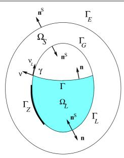
Fig. 1 Static equilibrium conf guration of a fuid-structure system for a compressible liquid with surface tension and sloshing effects
