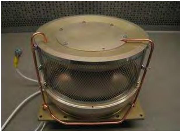
Fig. 1. Electrostatic analyser SWA-EAS for Solar Orbiter [source: D.O. Kataria and C. Owen from MSSSL].
