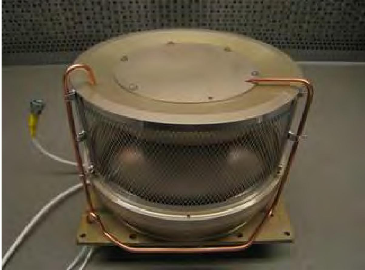
**Electrostatic analyzer SWA-EAS for Solar Orbiter -**
