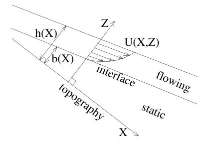
Figure 3: Steady flow with static/flowing transition, in the case when  $\theta$  is constant. The topography has slope angle  $\theta$ . The free surface and the interface have slope  $\mu_s$ , so that gravity balances internal friction within the flowing layer. The velocity profile is continuous across the interface, but not necessarily differentiable since the viscosity vanishes. The shape of the profile is arbitrary, and can be exponential for example, as it is often observed in experiments.
