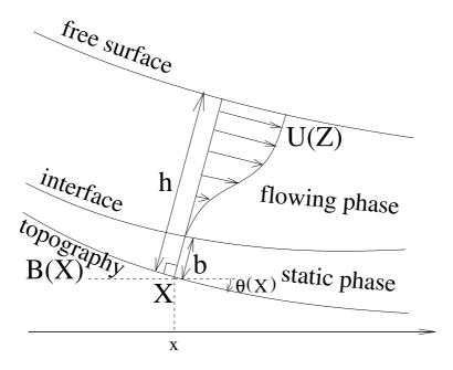
Figure 2: Generic velocity profile for viscoplastic flows with static/flowing interface. The tangential velocity U has a static part 0 < Z < b and a flowing part b < Z < h, separated by an interface b, where b is the thickness of the granular layer. The case b0 and b2 is represented.
