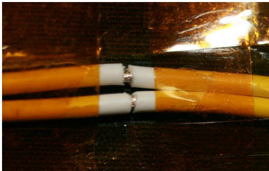
Fig. 10: Kapton film protection of substrate for IPG configuration
