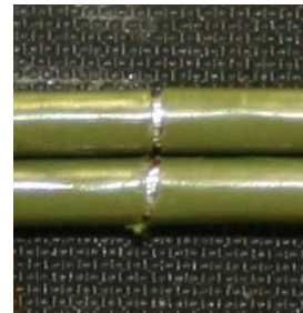
Fig. 3: pristine Kapton® cables. Cracks are made with cutter
