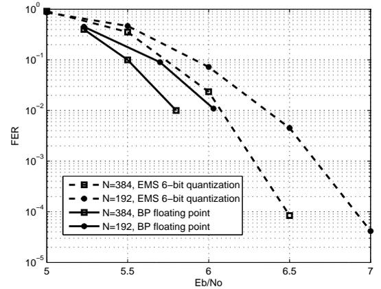
**Fig. 5** Performance comparison of the BP and EMS for a GF(64)-LDPC associated to a 64-QAM
