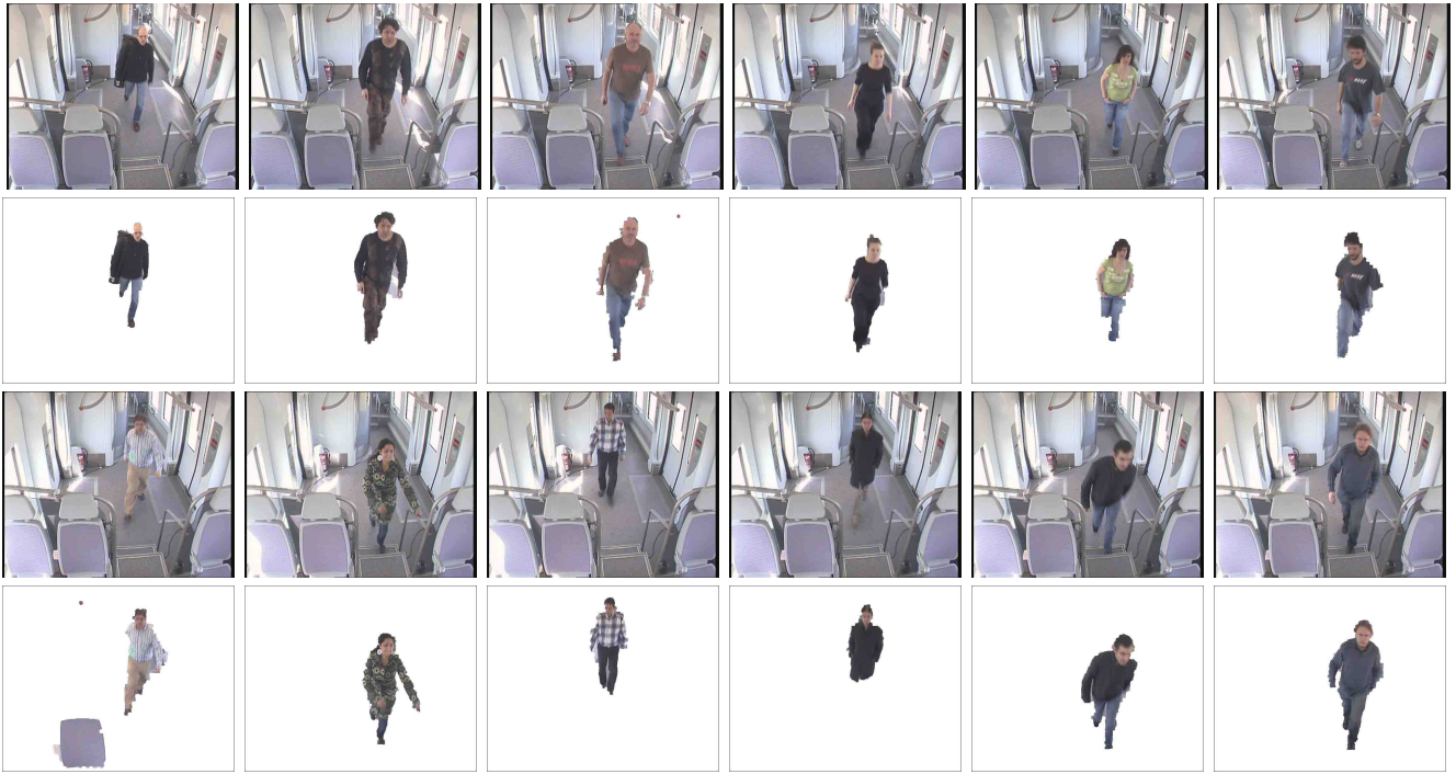
Fig. 4. People extraction: original images (lines 1 and 3), people extraction with the proposed method (lines 2 and 4).
