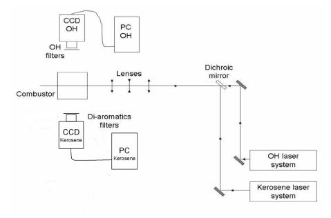
Fig. 8 PLIF apparatus for simultaneous measurements on kerosene and OH radical.
