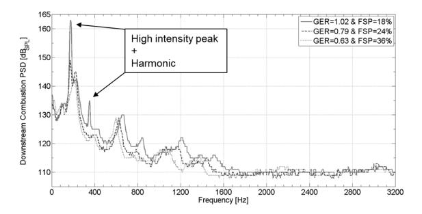
Fig. 4 Preliminary PSD measurements for stability mapping.
