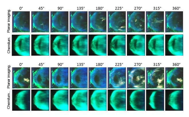
Fig. 6 Temporal sequence of instantaneous high-speed images of the spray planar imaging and the flame OH\* chemiluminescence for two flame behaviors : Upper : stable case IEL = 1955 mm ; Lower : unstable case IEL = 2405 mm  $(\dot{m}_{ar} = 100 \text{ g/s}; \text{GER} = 0.76; \text{FSP} : 4\%)$
