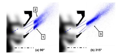
Fig. 11 Liquid kerosene spatial distribution at the outlet of the injection system for cycle phase angles of 90° (a) and 315° (b).
