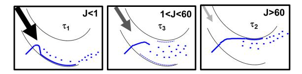
Fig. 12 Schematic scenario of the three different atomization phenomena depending on the momentum ratio between the liquid jet and the cross-flow.
