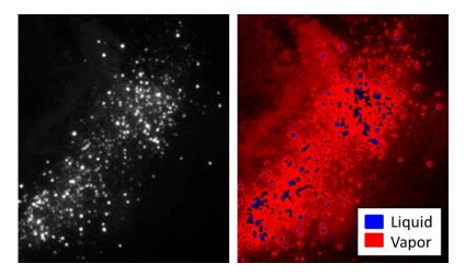
Fig. 9 Threshold processing on a sample image of PLIF on kerosene fuel revealing liquid (blue) and vapor (red) states.
