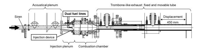
Fig. 2 Schematic of the LOTAR experimental setup.
