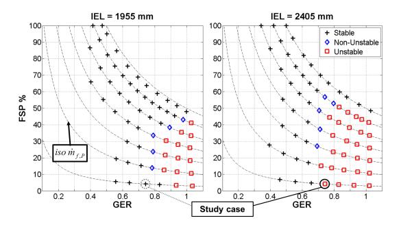
Fig. 5 LOTAR set-up stability map for IEL=1955 and 2405 mm, with  $\dot{m}_{air} = 100$  g/s,  $T_{air} = 473$  K.
