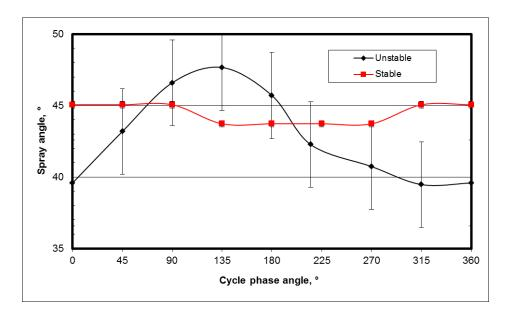
Fig. 7 : Spray angle oscillations during a thermo-acoustic instability cycle.
