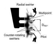
Fig. 3 Schematic of a novel aero-engine injection system used in the experiments.
