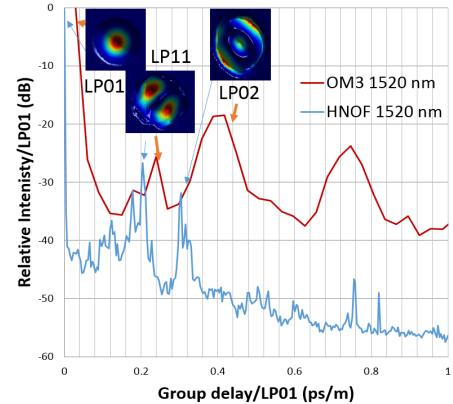
**Fig. 4:** Relative intensity of higher order modes of HNOF and OM3 fiber versus group delay difference referred to fundamental mode LP01. Associated transverse intensity profile of higher order modes LP11 and LP02
