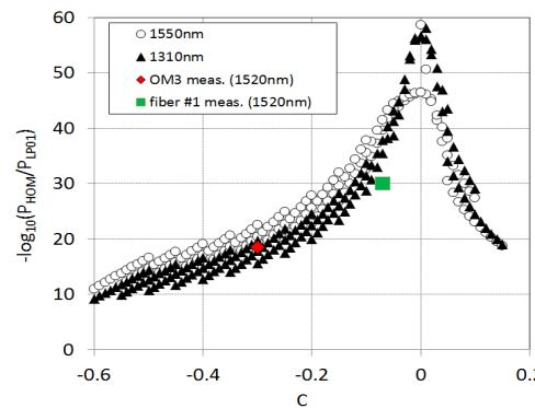
Fig. 1: HOM optical power over fundamental mode optical power in HNOF excited by a SMF
