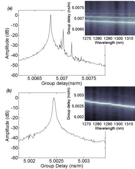
**Fig. 3:** OFDR reflectogram at 1310nm and group dispersion curve for (a) OM3 fiber (b) HNOF
