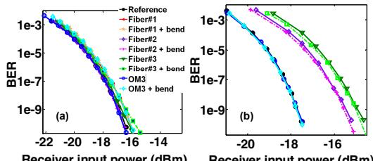
**Fig. 5:** BER measurements with 10 Gb/s NRZ signal on 100 m HNOF fibers and impact of bending constraints ( $R=1\text{cm}$ , 10 turns) : (a) single-mode, (b) multi-mode
