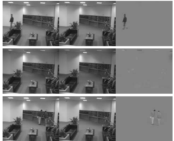
Fig. 4: Left: Original frames of a video sequence (300 frames). Middle and Right: recovered background (low-rank) and foreground (sparse) components.
