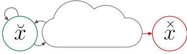
Fig. 3. The limit-cycle walker subject to perturbations as a state transition system. The cloud represents the set of states that are neither fall nor limit-cycle state.
