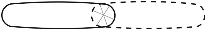
Fig. 6. For two objects in interpenetration (one in the plain line, one in the dash line), a degenerate case where there are an infinity of witness pairs, some of which are depicted in gray.
